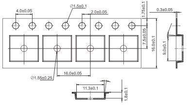
Cathode mark comes to feeding hole side. The direction shall be one in a reel.
